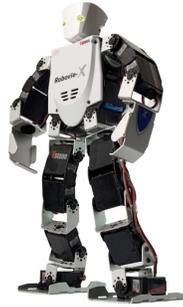
**Fig. 1.** The small humanoid used in this work: the Vstone Robovie-X.
