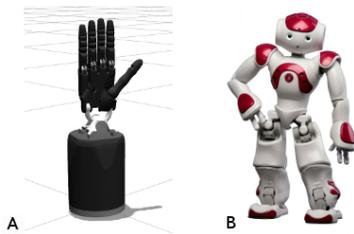
Fig. 5. Robots on which has been tested the framework: A) Simulated hand (Shadow Robot); B) Humanoid (Aldebaran NAO)
