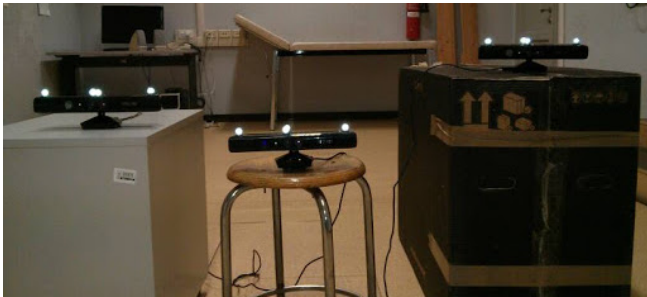
Fig. 4. One of the test scenarios. Four markers are placed on each Kinect in order to recover their locations by means of a motion capture system.
